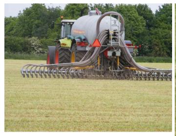
Reducing the surface area of applied slurry that is in contact with the air reduces ammonia emissions. This results in 20-25% more nitrogen being available to grass when using the trailing shoe compared to slurry being applied with a splash plate.
