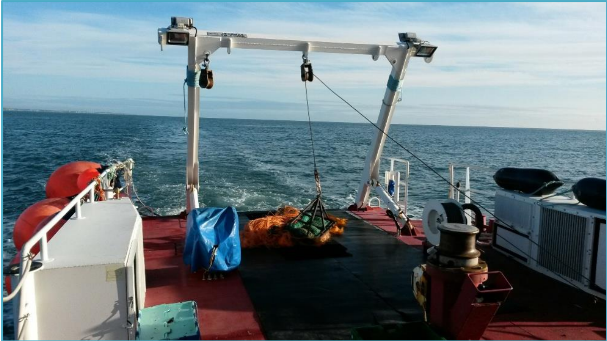
Figure 2: Photograph showing the dredge used during the Summer 2018 surveys.
