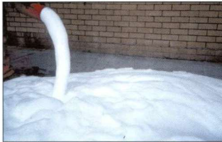
Figure 6 – Example of wet foam concrete from Good Concrete Guide 7, a report from the Materials Standing Committee of The Concrete Society
