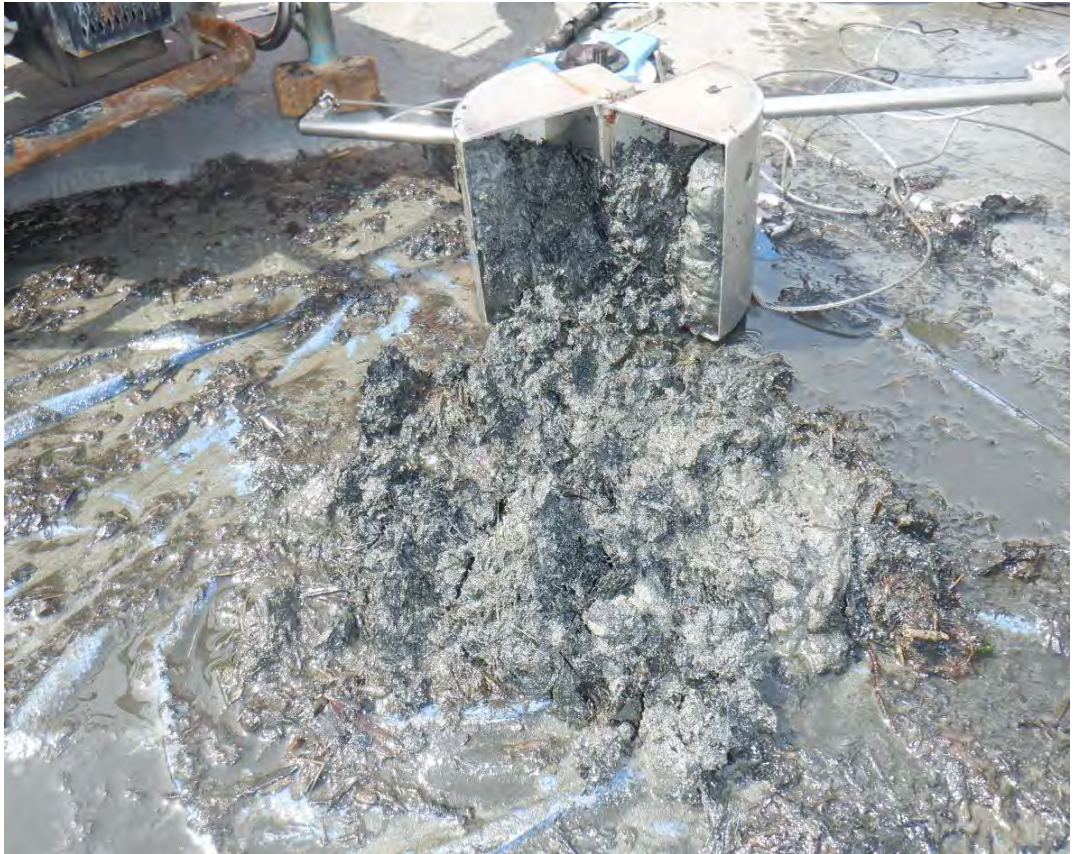
BC01 Van Veen Sediment Sampler Recovery
