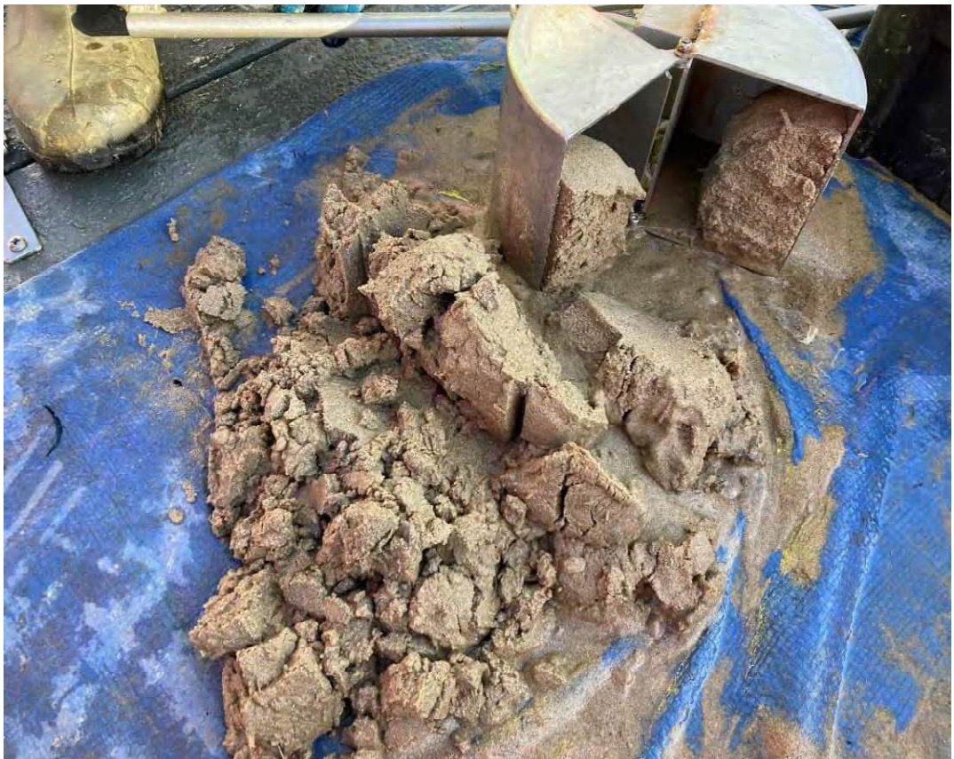
PR03 Van Veen Sediment Sampler Recovery
