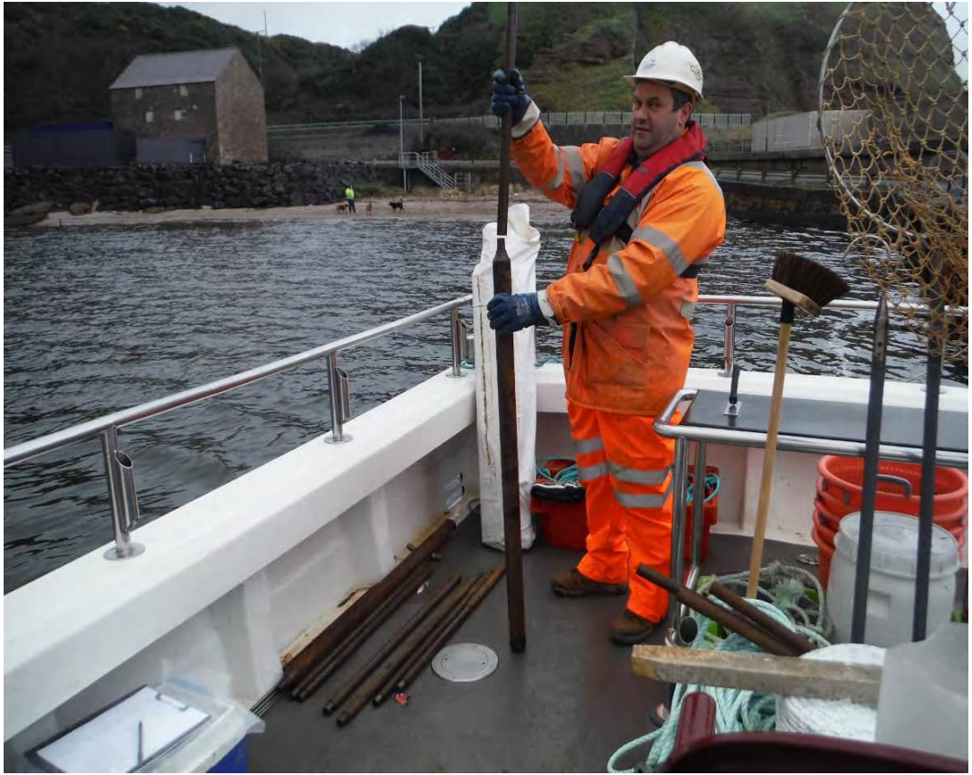
Dual Tube Sampler and Drill Rod
