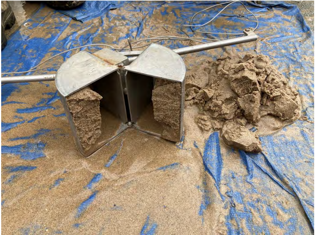
PR01 Van Veen Sediment Sampler Recovery
