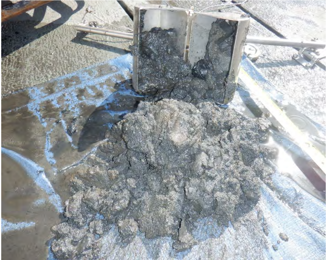
BC03 Van Veen Sediment Sampler Recovery
