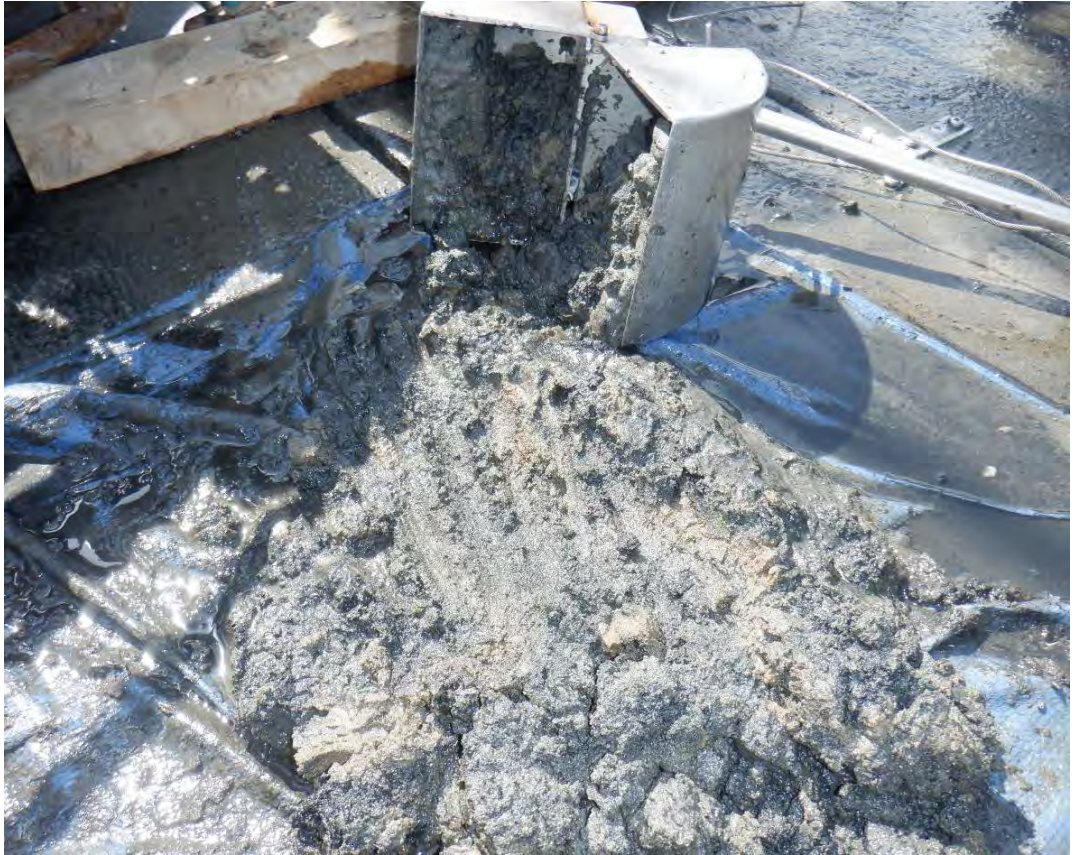
BC02 Van Veen Sediment Sampler Recovery
