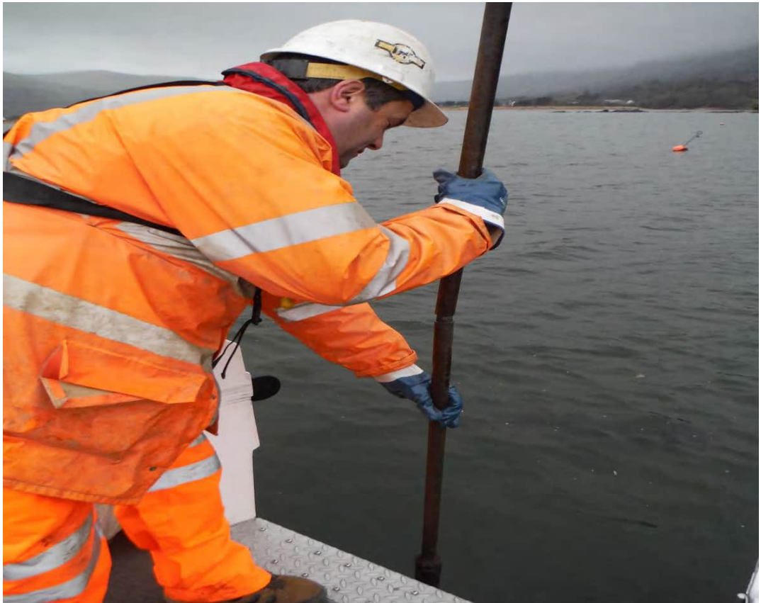
Dual Tube Sampler Lowered to Sea Bed. Additional Drill Rods Added as Required
