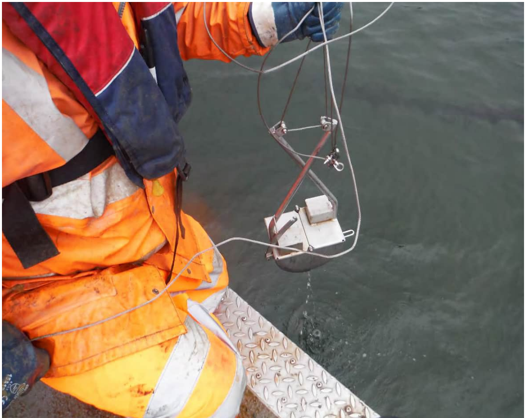
Recovery of Van Veen Sediment Sampler with Sample
