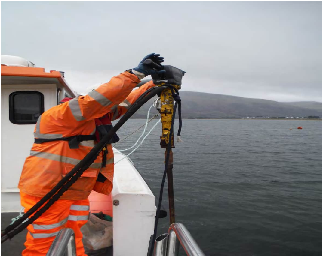
Dual Tube Sampler Driven into Sea Bed
