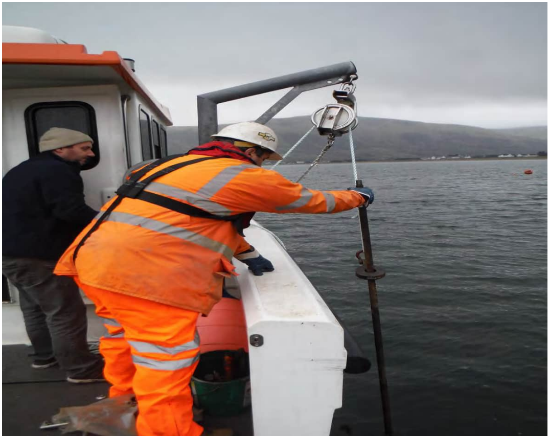
Recovery of Dual Tube Sampler Using Winch and Pulley System
