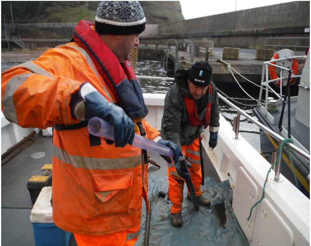
Insertion of PVC Liner into Dual Tube Sampler
