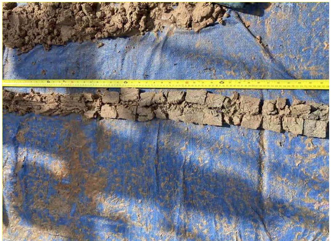
PR01 0m-2.0m Macro Core Sampler Recovery
