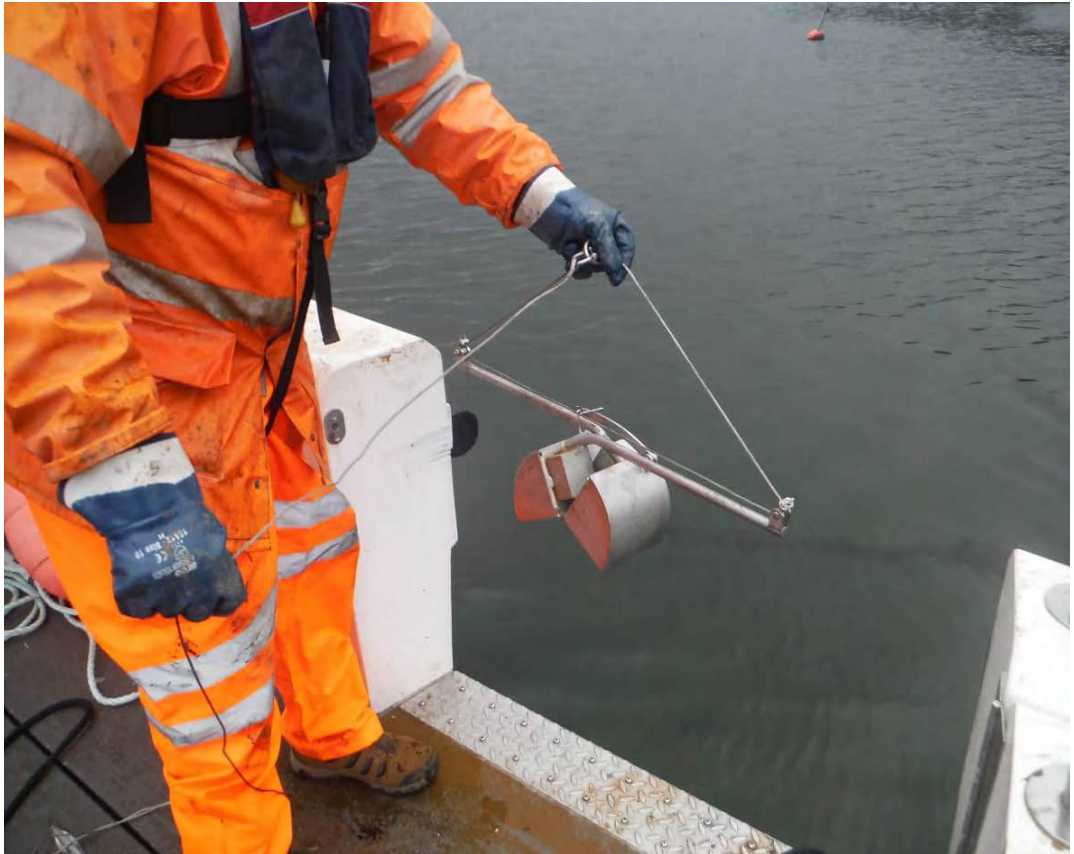
Van Veen Sediment Sampler Ready to be Lowered to Sea Bed
