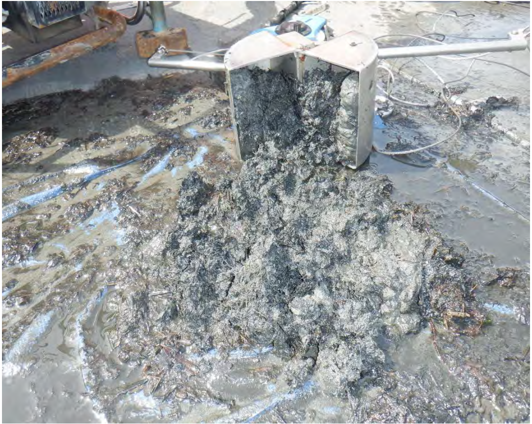
BC01 Van Veen Sediment Sampler Recovery
