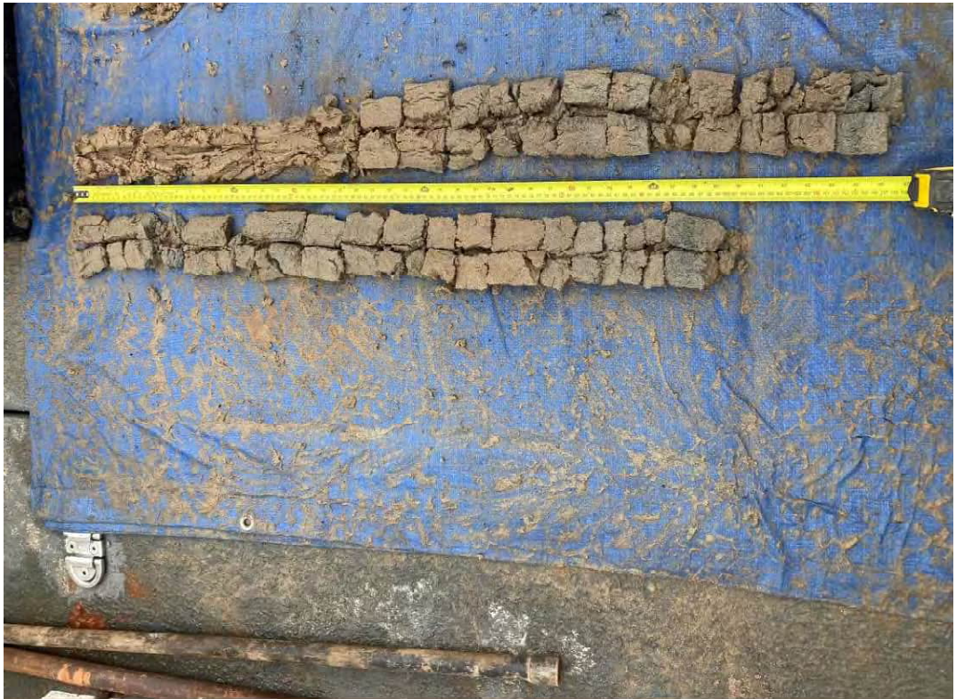
PR02 0m-2.2m Macro Core Sampler Recovery
