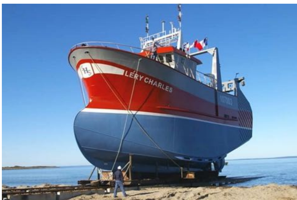
Figure 36 Modern fishing vessel showing deeper draught and keel. Source: Macduff Ship Design
