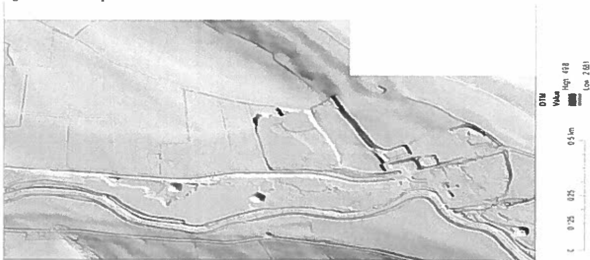
Fig 11 - Mobouy DTM2. shows the relief in the Mobouy site, hill shaded to highlight the topographic features such as drains, the river, banks and pylon foundations.
