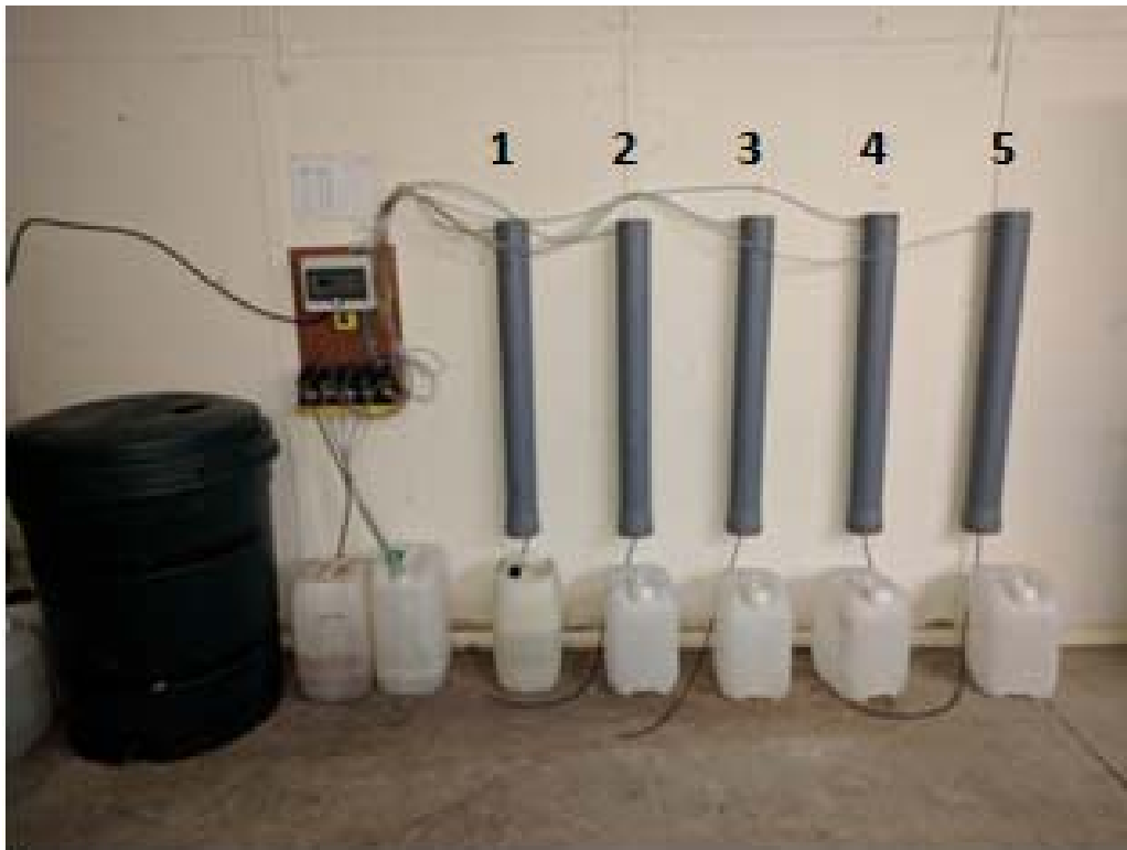
Fig 2 – The Column testing equipment testing continual leachate application
