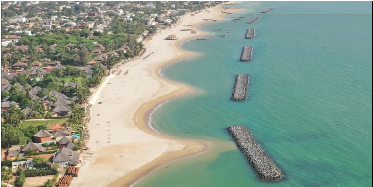
Figure 3.10: Example of offshore breakwaters with salient and tombolo formations.
